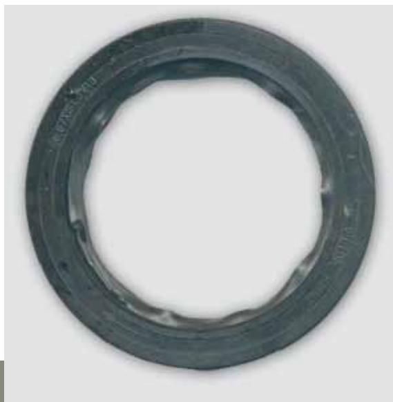
▲ Damaged PTFE sealing lip as the cause of failure.
