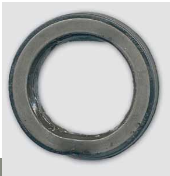
▲ Greased PTFE sealing lip as the cause of failure.
